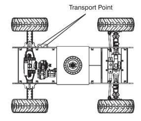
Figure 3-3a. Turret Transportation Lock & Locking Points (Models SJ46AJ & SJ51AJ)
