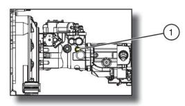
Figure 2-7b. Drive Bypass Valve (Model SJ63AJ)
