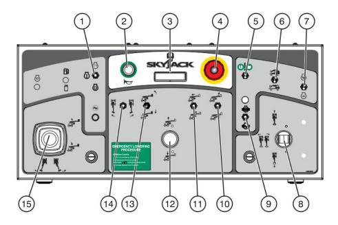
Figure 2-6. Platform Control Console
