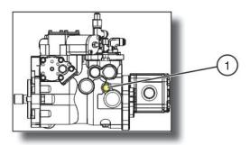
Figure 2-2a. Drive Bypass Valve (Models SJ46AJ & SJ51AJ)
