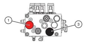
Figure 2-8a. Brake Manifold (Models SJ46AJ & SJ51AJ)
