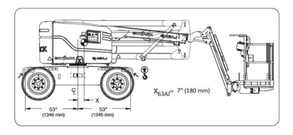
Figure 3-3d. Lifting Points (Model SJ63AJ) NOTE: Center of gravity varies with different options.
