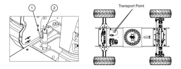
Figure 3-3c. Turret Transportation Lock & Locking Points (Model SJ63AJ)
