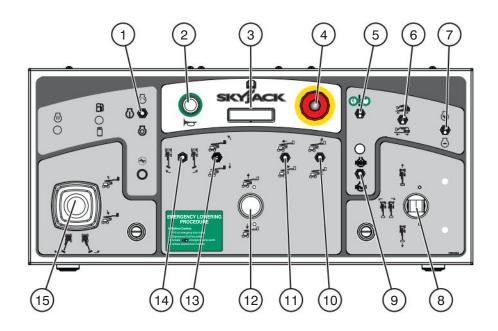
Figure 2-6. Platform Control Console
