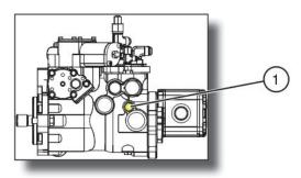
Figure 2-7a. Drive Bypass Valve (Models SJ46AJ & SJ51AJ)
